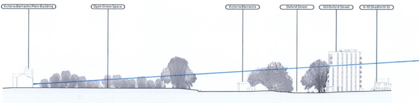
Cross Section showing view of proposal from Main Barracks building – the upper 2-3 storeys will be visible, and more in winter from GBA EPBC Self Assessment, blue view line added
